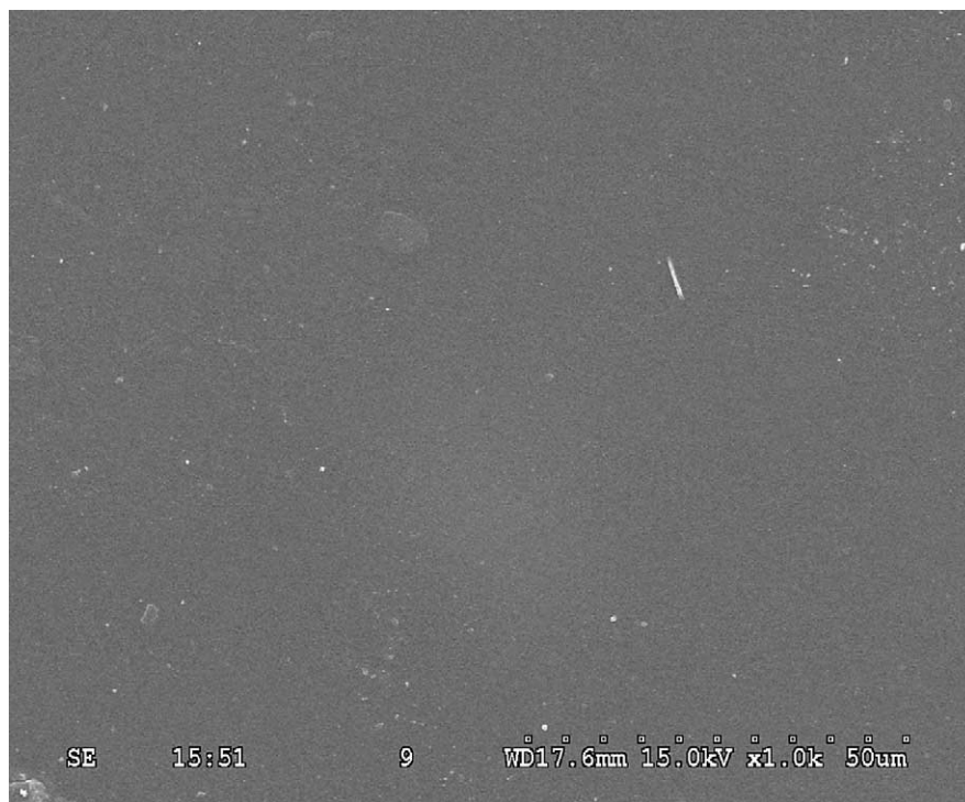
Fig. 1. Scanning electron micrograph of alkaline PVA-PECH (1:0.2) SPE.
